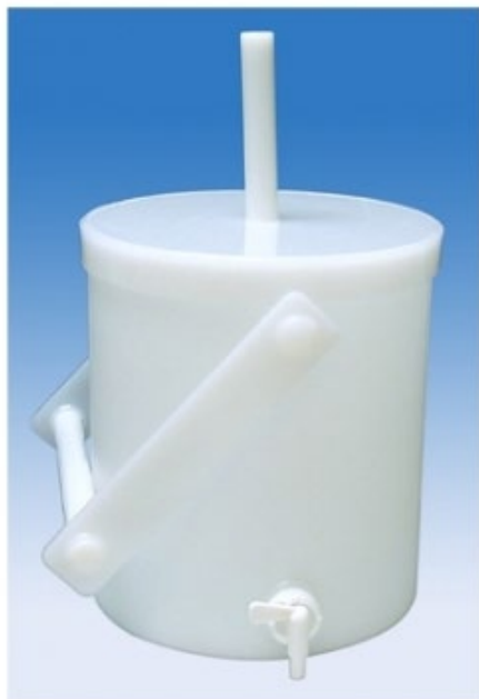
Figure 5. Image of a 15-liter churn splitter used during the laboratory comparison exercise ( Source of photograph: https://shop.sciencefirst.com/wildco/general-laboratory-equipment/6178-churn-sample-splitter-polyethylene-14l.html )
