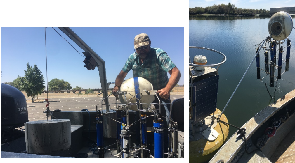
Figure 3. Photos of water-quality instrument deployments at the Mossdale at San Joaquin River (left) and Liberty Island at Cache Slough (right) stations. Sensors were deployed at the same water depth relative to the surface at both locations (~1 m). Instruments were attached to a stainless-steel cage for both two week deployments. Left photo shows Mike Dempsey (DWR) with the instrument cage is attached to both a concrete weight and surface marker by a \frac{3}{8} -inch stainless-steel cable that creates the taut-wire mooring. Right photo is the instrument cage connected to the continuous monitoring buoy with a stainless steel cable and a six-foot aluminum pipe to maintain separation between buoys.
