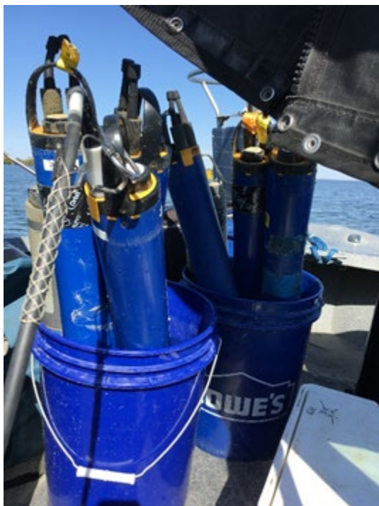
Figure 4. Bucket test of sondes following sensor intercomparison deployment.
