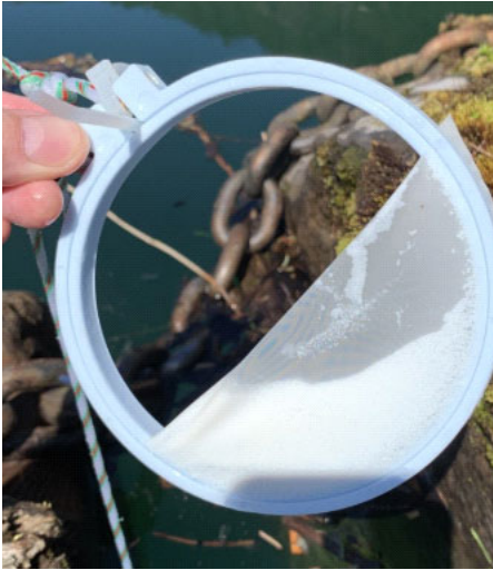
Figure 3: Photo showing the planned system for deploying SPATT at fixed locations.
