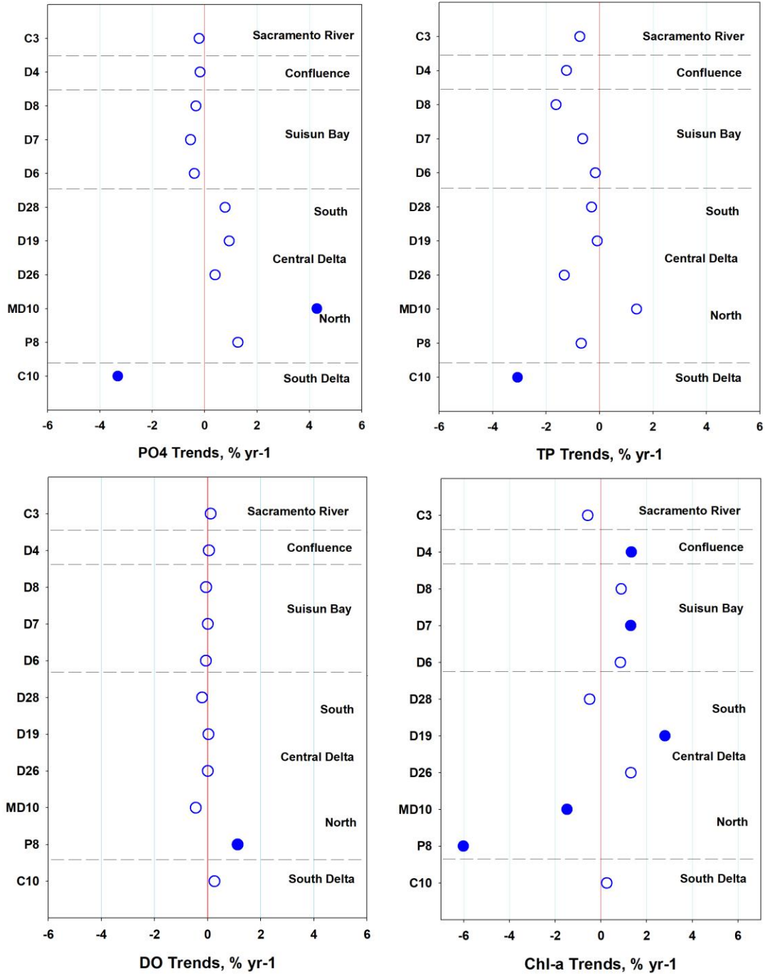
Figure 31. Magnitude (% change per year) of detected trends at DWR-EMP stations, WY 2001–2016 data (significance at p \leq 0.05 ), for PO_4 , TP, DO, and Chl-a.
