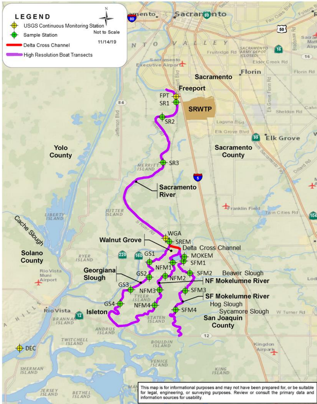
Figure 1. Map of the Sacramento-San Joaquin River Delta showing project sample stations in the lower Sacramento River, Georgiana Slough, North Fork Mokelumne River, and South Fork Mokelumne River, showing high resolution boat mapping transects (purple lines) and the Delta Cross Channel (red line). Yellow circles denote USGS continuous monitoring stations. Green circles denote sample stations.
